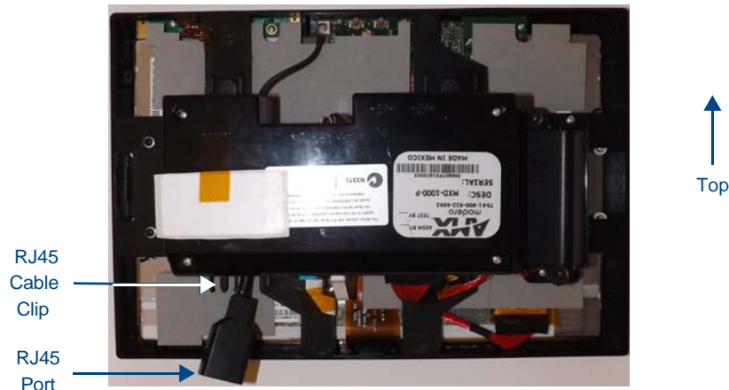
FIG. 18 Rear of the MXD-1000 (detail of the RJ45 connection)
